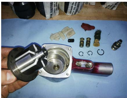
PNEUMATIC MOTOR REPAIR
