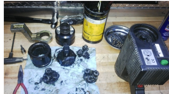
ELECTRIC GEARBOX REPAIR
